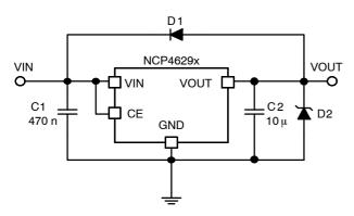
Figure 4. Typical Application Schematic with Protective Diodes
