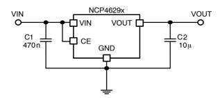
Figure 1. Typical Application Schematic
