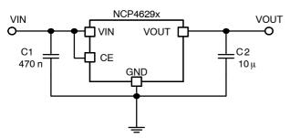
Figure 3. Typical Application Schematic
