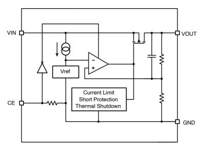
Figure 2. Simplified Schematic Block Diagram
